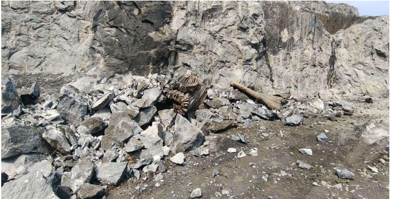
Fig 17: Fragmented Rock after Blasting
