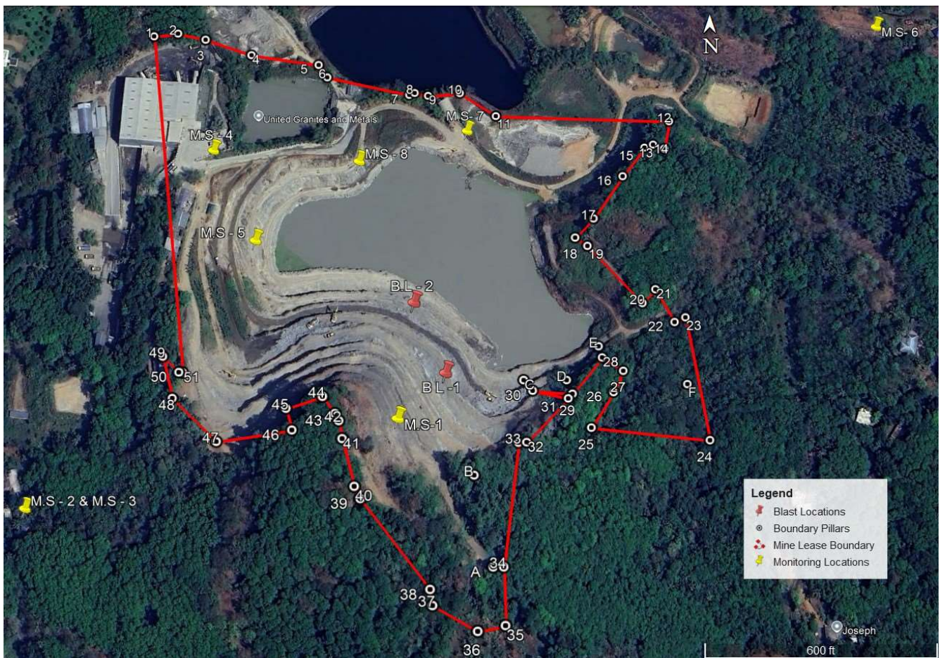
Fig 4: Google Earth Image of the Mine showing Blasting Locations & Monitoring Points
