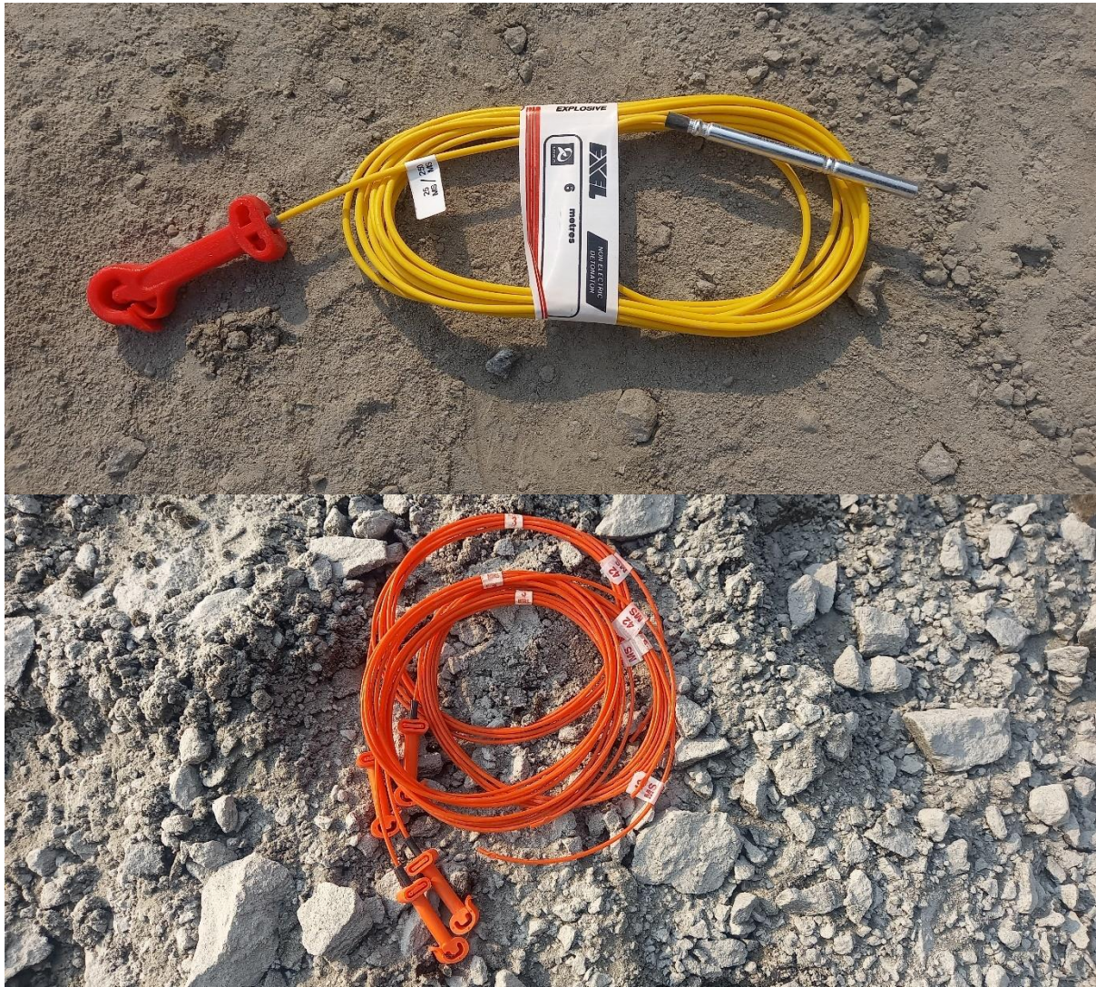
Fig 7: Non-Electric Detonator & Surface Trunk Line Delay used in the Quarry
