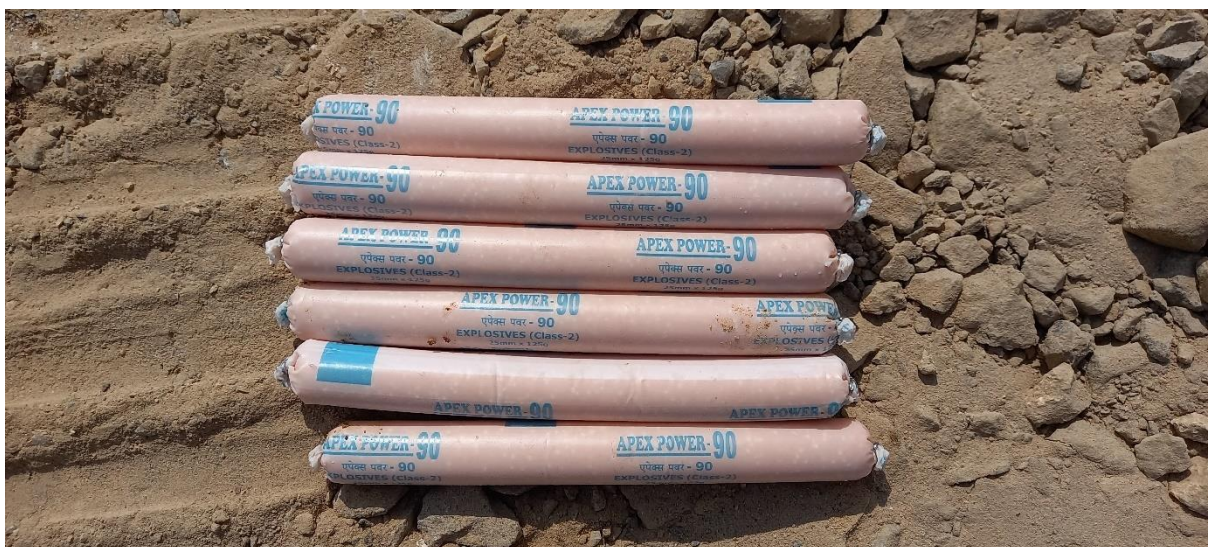
Fig 8: Explosive Cartridges used in the Quarry
