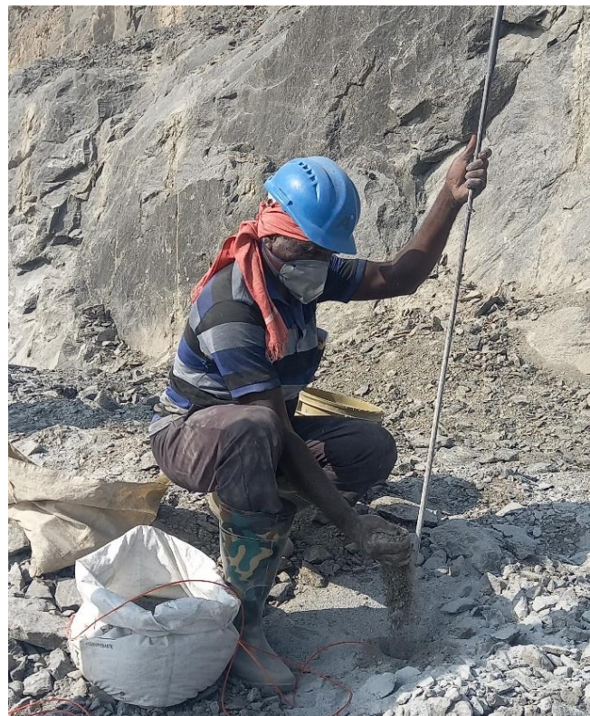
Fig 11: Stemming of Blast holes
