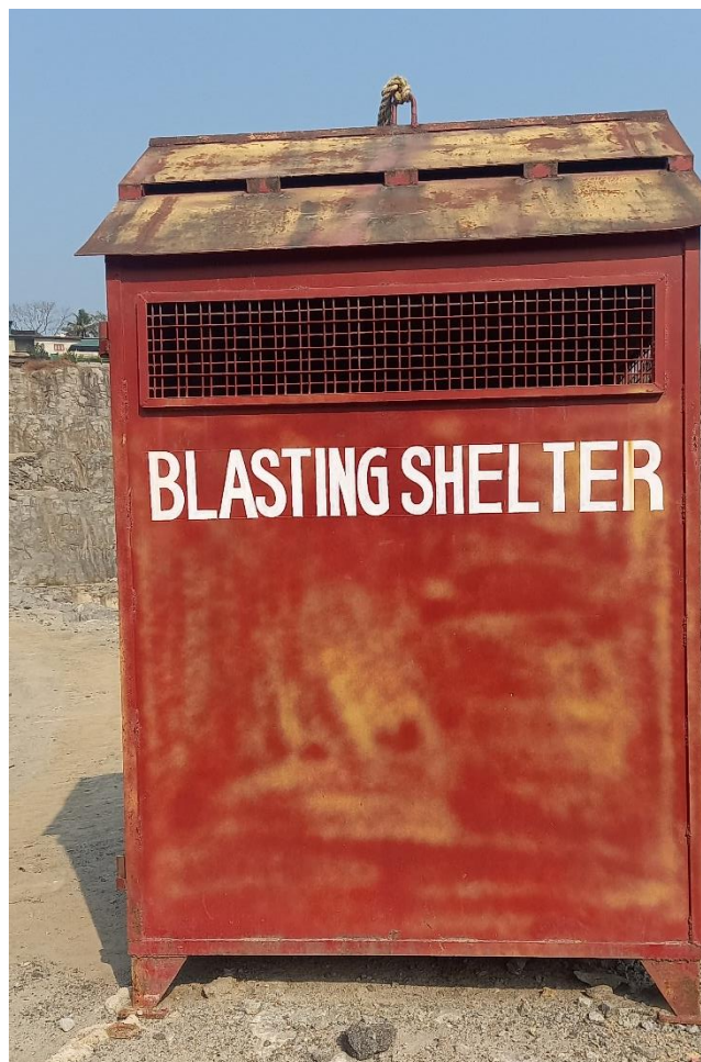
Fig 16: Blasting shelter for Safety of Blasting Personals
