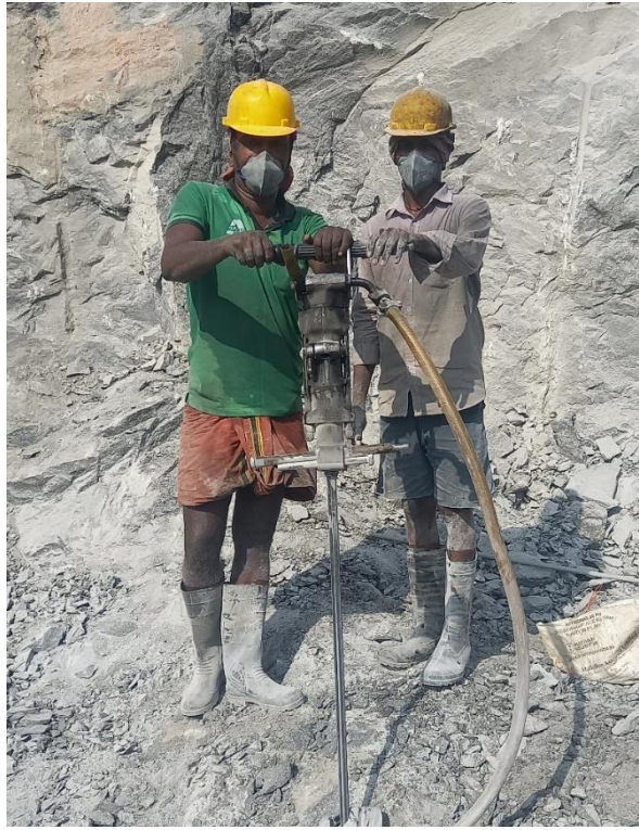
Fig 6: Drilling of blast holes using jack hammer
