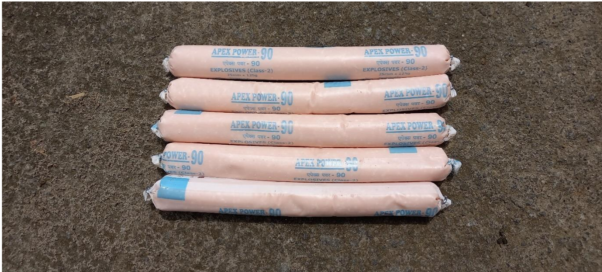
Fig 8: Explosive Cartridges used in the Quarry
