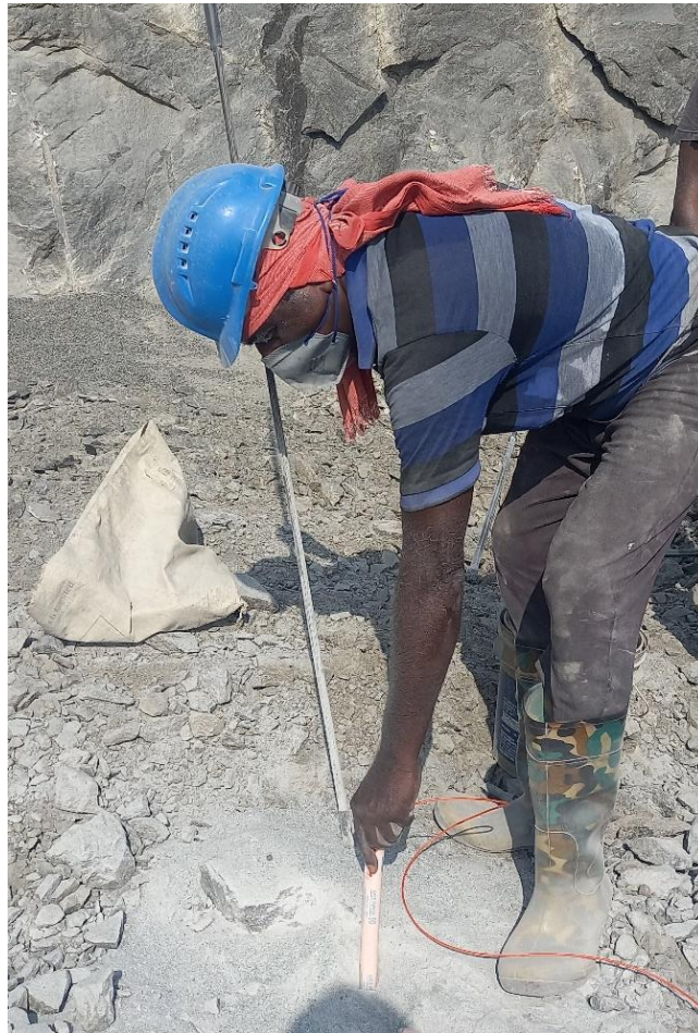
Fig 10: Charging of Blast holes
