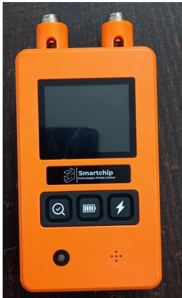
Fig 9: Initiator used to fire Electronic Detonator
