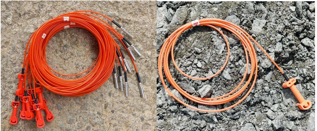
Fig 8: Non-Electric Detonator & Surface Trunk Line Delay used in the Quarry
