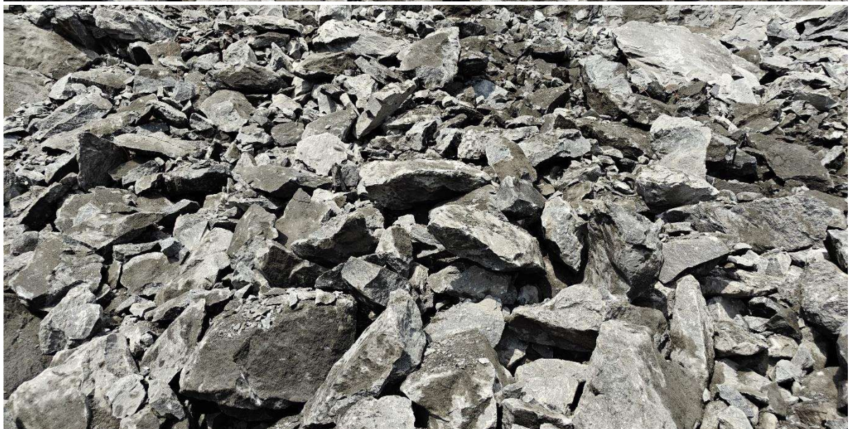
Fig 15: Fragmented Rock after Blasting
