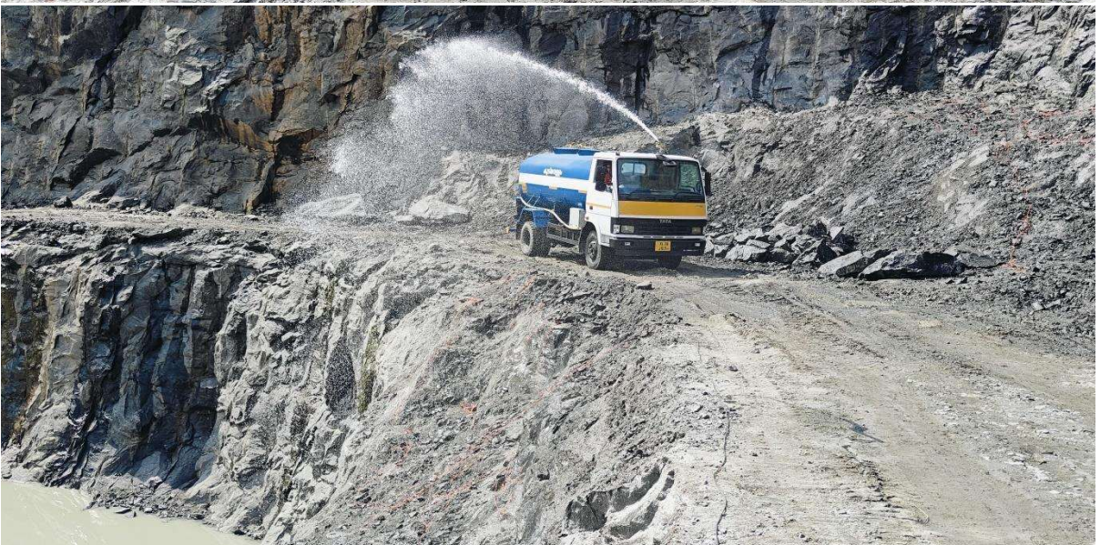
Fig 13: Water spray system
